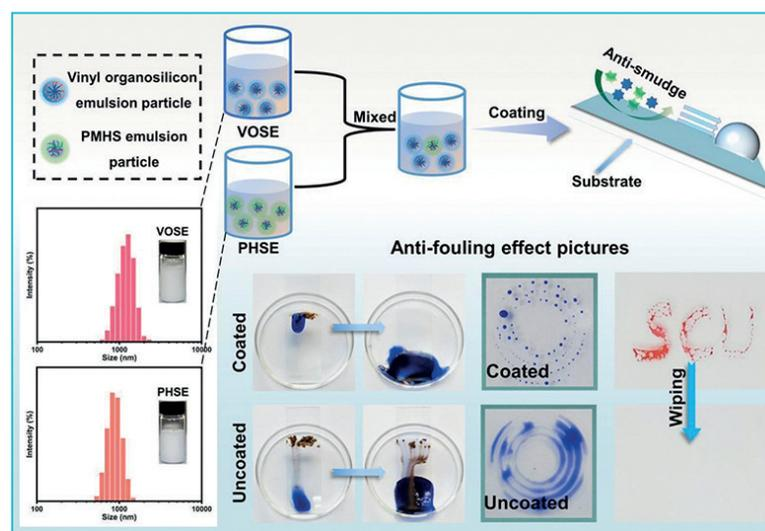
surfactants for emulsification of vinyl organosilicon components and polymethylhydrosiloxane (PMHS), respectively.
