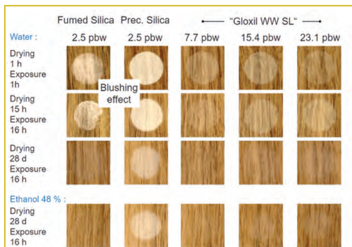
Fig. 2 - Resistance properties of matted coatings against water and diluted alcohol exposure at early stage and after 28 d of drying, DFT 105 \mu\text{m} (3 x 35 \mu\text{m} )
