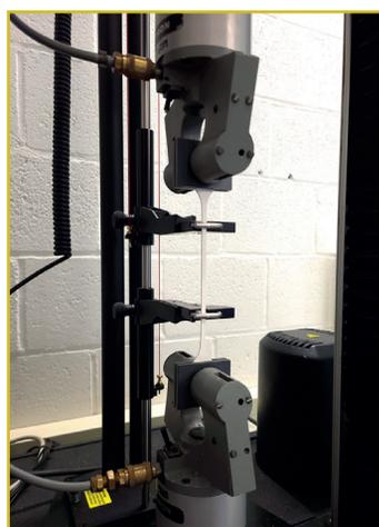
**Fig. 5 Polyresyst® IC6005 shown during an elongation test**
