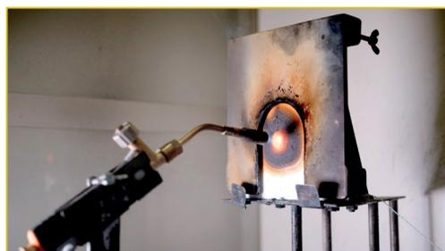
**Fig. 2 Front side steel substrates with Polyresyst® IC6005 exposed to a 1100-degree Celsius flame**
