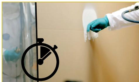
**Fig. 4 Polyresyst® IC6005 sprayed on cardboard, cures in just a few seconds**
