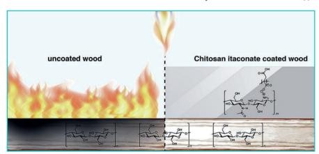
and a sustainable alternative to steel and concrete in construction. However, wood generally needs protection from a number of external influences such as moisture, UV, stains, and also fire. Fire poses a particularly great danger to wood structures. Due to its chemical structure untreated wood can easily ignite, and once burning, it tends to sustain combustion until it is completely consumed, even without an ongoing external heat source.
